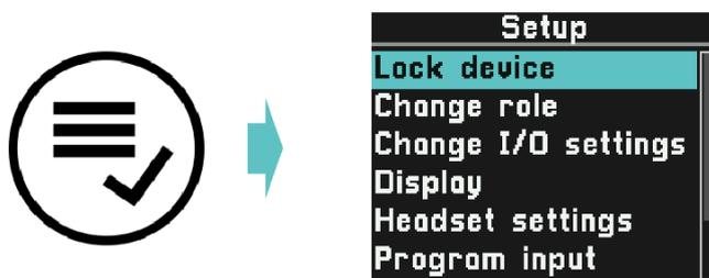
Role settings for your device may include an option to lock the front panel using a 4 digit pin. The pin is defined per Role in Q-Tool configuration software.
