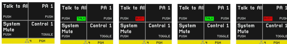
The assigned function can be activated by pressing the TALK or the CALL button near the quadrant.
