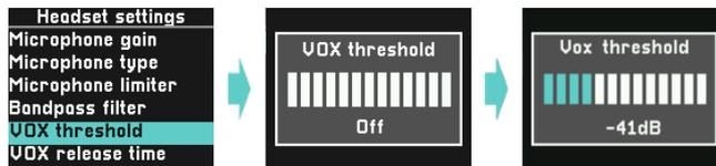
The Vox function acts as a signal gate and is used to reduce background noise in the system. The Vox threshold level determines at which level an audio signal is passed on to the system. Setting the Vox threshold to off completely removes the gate function from the signal path.
