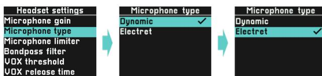
Electret microphones require a bias voltage for correct operation. If you set the microphone type to electret, a bias voltage will be applied to the microphone input. Dynamic microphones work without bias voltage.
