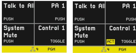
Control outputs are part of the Q210P Speakerstation product, but can be controlled from any device in the system. If the output is active you will see a yellow ACT indicator.
