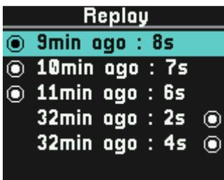
By pushing either of the Replay buttons on top of the Beltpack, the last recorded message will be played back immediately. Use the Replay buttons on top of the Beltpack to scroll through the list. You can see how long ago each message was recorded, how long each recorded message is and the dot shows which Channel each
