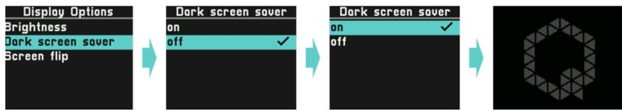
If the Dark Screen Saver is enabled, it will be activated automatically and deactivated by any button press or encoder turn. It will show a very low brightness Q logo when active.
