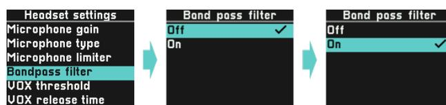
A Band Pass filter removes lower and higher frequencies from your microphone signal to improve speech intelligibility. Set to on if desired.
