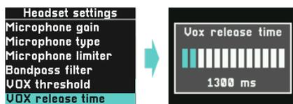
Vox release time determines how long your speech signal will be passed on to the system once the signal level goes below the VOX threshold level. This is used to avoid chopping your speech. VOX release time can be set from 500 milliseconds to 5 seconds in steps of 100 milliseconds.
