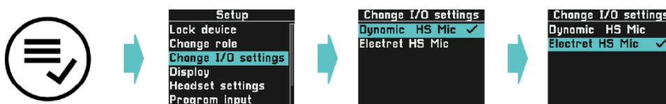
Select from different Headset settings presets. Q-Tool configuration software allows to define more I/O settings to match the specifics of the Headset of your choice.
