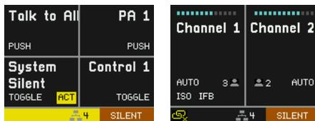
System silent stops the speaker of the Q210P Speakerstation and any other (future) devices from making sound. Public announcements remain functional, optical signaling when using a CALL function remains functional as well. The function is activated through a button push. Pressing the button again deactivates the function (TOGGLE behavior). If system silent is active, you will be notified by an orange SILENT indicator.
