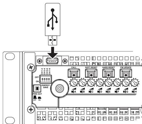
3. Keep pressed the FW UPDATE pushbutton until the front LED bars start blinking.
