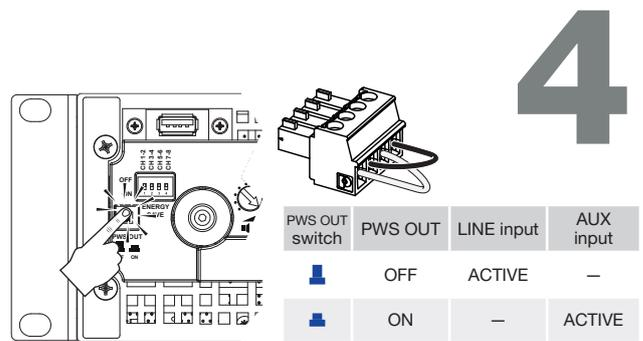
FIG. 3: Manual procedure to switch from LINE to AUX.
