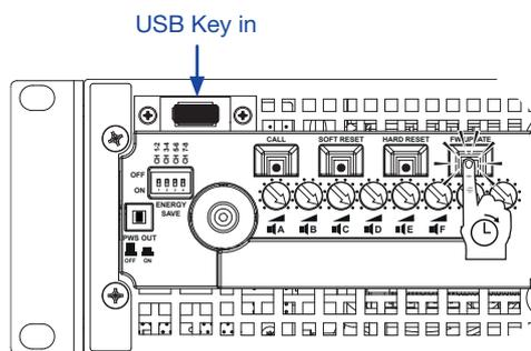
4. The update process lasts in 3-5 minutes. At the end the system reboots and it is possible to extract the USB storage device.
