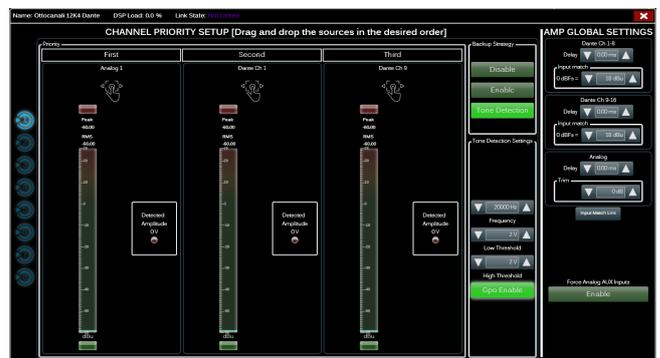
FIG. 4: Ottocanali DSP+D: Input selection and backup policy.
