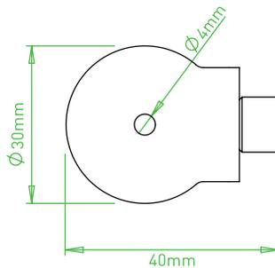
**Pro Cable Connector** - Power and data integrated in a single cable with 5-pin, sealed, locking connector. For use with our G8 Distribution Box and Pro Cable system.
