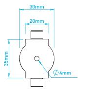
**Pro Cable Connector** - Power and data integrated in a single cable with 5-pin, sealed, locking connector. For use with our G8 Distribution Box and Pro Cable system.
