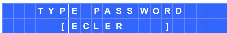
Using an encoder (ZA to ZB), edit the selected character, and using the PARAMETER key, select the next character to edit. Finally, press SHIFT + ENTER to validate the entered password.
