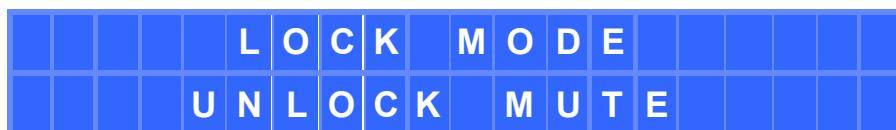
Using the rotary control, it is possible to change the desired locking mode and then press SHIFT + ENTER to confirm the selection. If you select one of the three password protected modes (LOCK ALL, UNLOCK OUTS or UNLOCK INS&OUTS), the next screen prompts you to enter the lock password:
