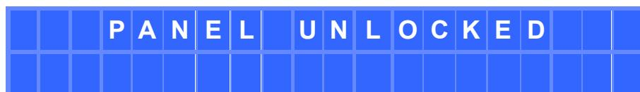
The equipment will be temporarily unlocked, until it remains 2 minutes without any activity on the front panel or returns to the lock menu (left and right MENU simultaneously for 2 seconds) to confirm or modify the lock mode, in which case it will go back to the password request (the same or a new one), which will be active starting from your validation (SHIFT + ENTER).
