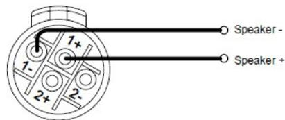
Additionally, the channel 2 output is duplicated on the Speakon™ connector for amplifier channel 1 for Bi-Amp wiring. Similarly, the channel 4 output is duplicated on the Speakon™ connector for amplifier channel 3. This can be useful for making a connection to two loudspeakers with one 4-core cable (i.e., Bi-Amp).
