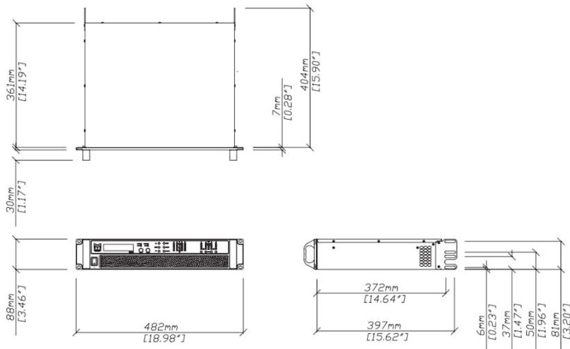
The iK42/iK81 Series Amplifier system is designed to be mounted in a standard 19" rack enclosure.
