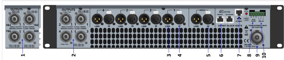
1. Loudspeaker Connectors (iK81). The amplifier Speakon™ outputs. Connect the first loudspeaker to the 1+ and 1- terminals and the second loudspeaker to the 2+ and 2- terminals. For Bridged mode, use terminals 1+ and 2+.
