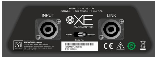
The XE300 may either be bi-amped or driven by a single full-range amplifier. For full-range use, it uses an internal crossover at a frequency of 1.1 kHz. The two modes of operation are selected by a switch on the front connector panel.
