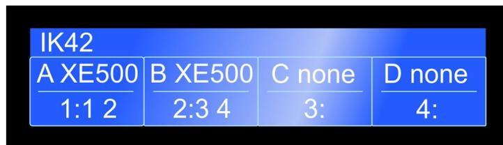
This shows that DSP A and B are both loaded with the XE500 preset. Input 1 is routed to output 1 & 2, input 2 is routed to outputs 3 & 4, output 3 and 4 are not used therefore not routed anywhere. The amplifier is ready for use.
