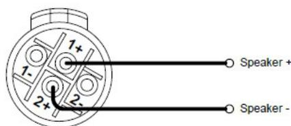
More than one speaker can be connected to each channel provided the total impedance per channel is not less than **2 ohms**. In bridged mode the minimum total impedance should not be less than **4 ohms**.
