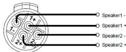
In addition, the channel 1 or channel 3 connector (all the Speakon™ connectors on the iK81 model) can also be used if the pair of amplifier channels is being operated in bridged mode.
