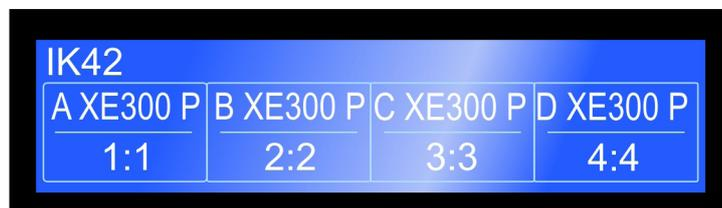
This shows that DSP A, B C and D are loaded with the XE300 Passive Preset, Input 1 is routed to Output 1, Input 2 to Output 2 and so on. The amplifier is ready to use.
