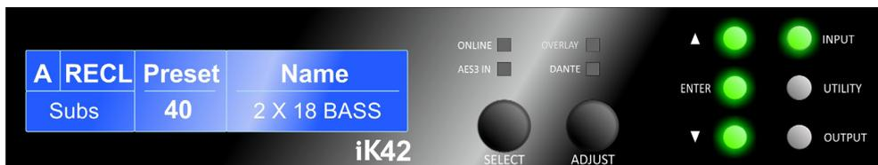
3. Use the **ADJUST** control to scroll round to the required XE300 Preset:
