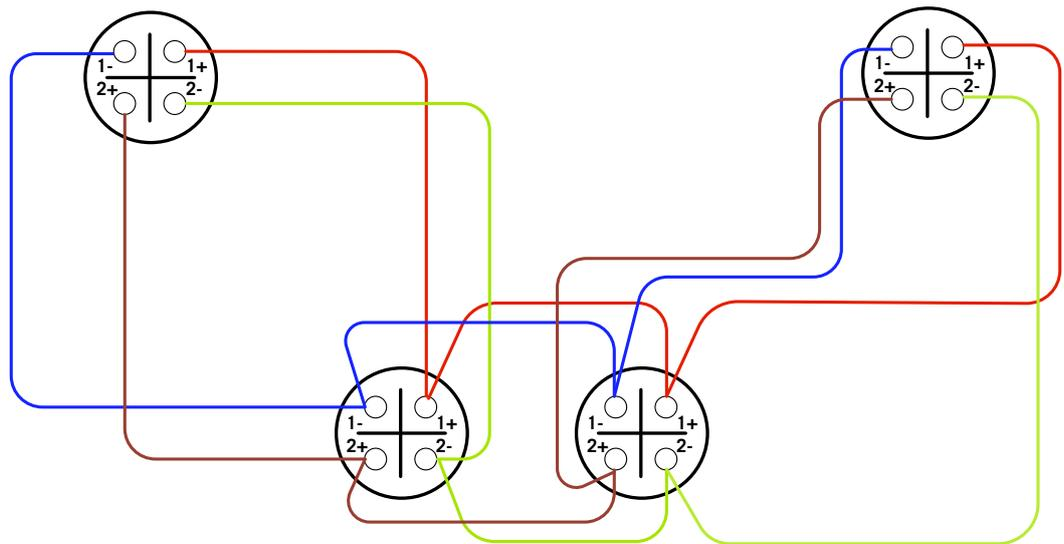
**Important:** Each iK42 amplifier channel can drive a maximum of two XE Series monitors in parallel. Do not attempt to connect more than two monitors to any one amplifier channel as the combined load impedance will be lower than the minimum impedance the amplifier is designed to drive. This will result in unsatisfactory performance and may cause damage to the amplifier.
