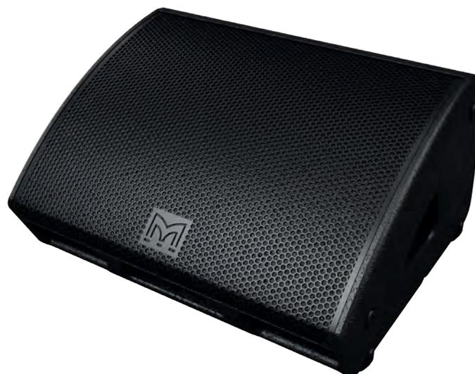
The XE300 is the definitive, high-performance compact monitor. It features a high-specification 12" (300mm) LF /1.4" exit HF Coaxial Differential Dispersion driver to deliver perfect sound over the artist's listening plane. The LF driver section has a 3" (75mm) voice coil and efficient motor with an aluminium demodulating ring to minimise distortion, while the HF driver utilises a 1.4" (35mm) exit HF compression driver with a 3" (75mm) pure titanium diaphragm.
