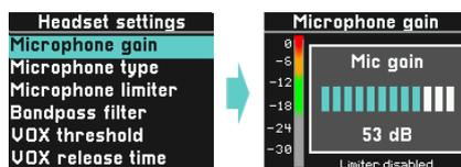
The gain of your microphone can be adjusted from 0 dB to 67 dB. Speak into your microphone at the volume you typically use when working and adjust the level to be in the upper green range.
