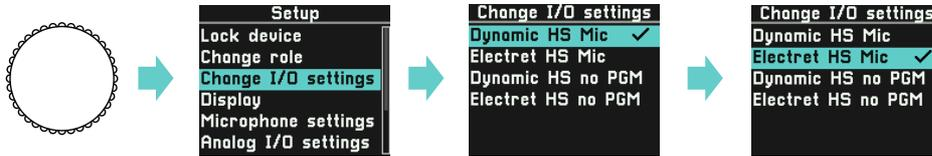
Select from different I/O settings presets. Q-Tool configuration software allows to define more I/O settings to match the specifics of external devices connected to your Speaker Station.
