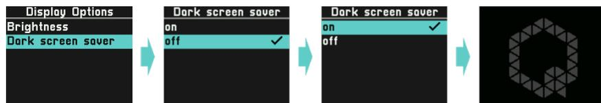
If the Dark screen saver is enabled, it will be activated automatically and deactivated by any button press or encoder turn. It will show a very low-brightness Q logo when active.
