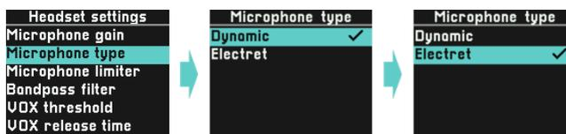
Electret microphones require a bias voltage for correct operation. If you set the microphone type to electret, a bias voltage will be applied to the microphone input. Dynamic microphones can work without bias voltage.
