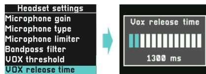
Vox release time determines how long your speech signal will be passed on to the system once the signal level goes below the VOX threshold level. This is used to avoid chopping your speech. VOX release time can be set from 500 milliseconds to 5 seconds in steps of 100 milliseconds.
