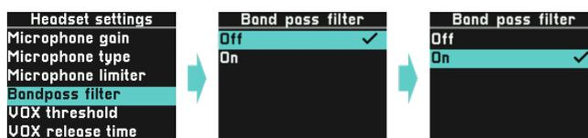
The Band pass filter removes lower and higher frequencies from your microphone signal to improve speech intelligibility. Activate it if needed.
