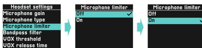
The limiter function is used to avoid distorted signals if someone gets excited and starts to speak more loudly. We recommend to set the limiter to on.
