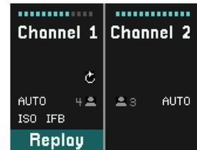
The Speaker Station's right display informs about how long ago each message was recorded and how long each recorded message is. Start playback of each individual message by pressing buttons A to C. The bottom line tells you which Channel the message was recorded from and indicates the volume setting. While playing back you may use the Channel volume encoder or the main rotary encoder to adjust the Channel volume.
