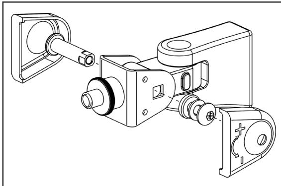
In order to fit the adapter to the monitor mount, you should first remove the installed screen bracket. To do this, pull off the two plastic covers on the monitor mount. Unscrew the screw underneath with the provided Allen key and remove screw and washers. Hold the screen bracket and remove the bolt.
