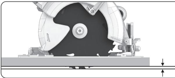
Adjust the cutting depth to the thickness of the workpiece. Less than a full tooth of the blade teeth should be visible below the workpiece.
