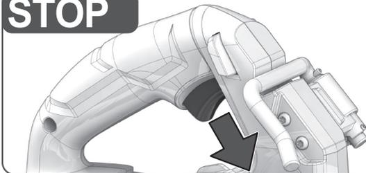
For safety reasons this power tool is fitted with a switch lock and the On-/Off switch cannot be locked in the „On“ position.
