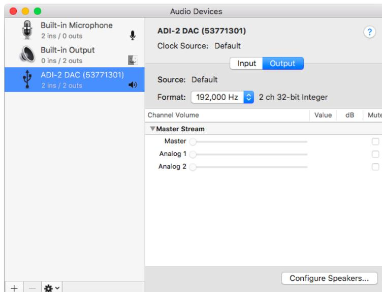
Applications that don't support card or channel selection will use the device chosen as **Input** and **Output** in the **System Preferences – Sound** panel. This setting is also available in the Audio MIDI Setup via the gear symbol at the bottom of the window.
