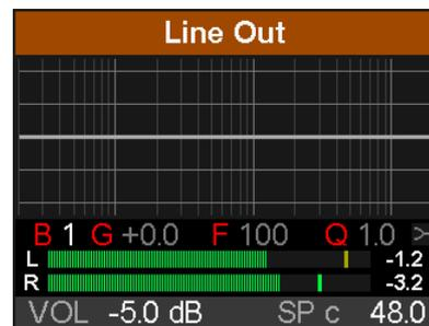
The graph has 5 different colors matching the 5 bands that can be adjusted. If the line is just grey the EQ is disabled (bypass). The EQ can be enabled in the second menu which comes up by pushing the EQ key a second time.
