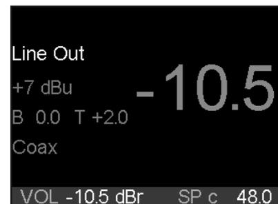
Despite this screen having no level meters, overloads caused by Volume, PEQ or Bass/Treble are easy to recognize. The big volume number is coupled to the over detection of the analog outputs. It changes its color to red when overloads occur.
