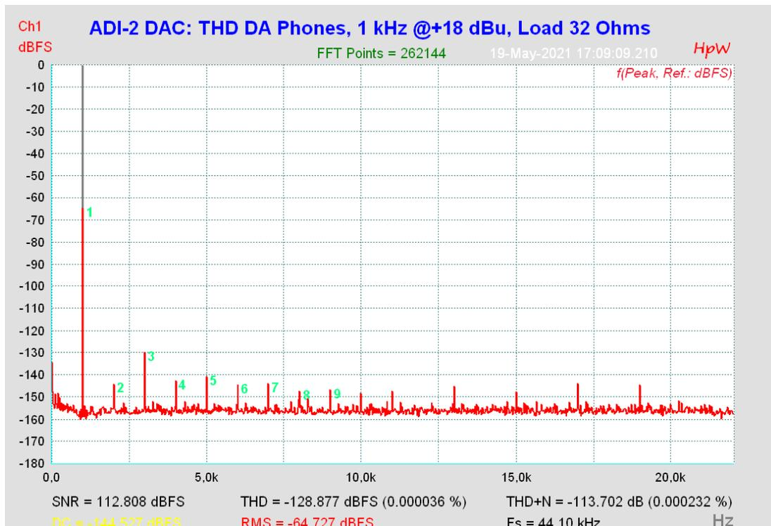
\* Measured with active notch filter via ADC of ADI-2 Pro FS
