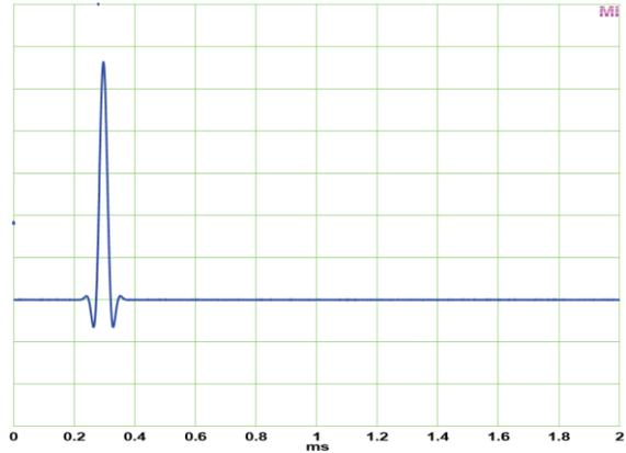
The screenshots above show the analog output signal of the DAC filters, stimulated by a digital single sample impulse at 44.1 kHz sample rate. While Slow has the most perfect response, it loses around 1.2 dB already at 15 kHz, see chapter 31.4. Both Short Delay are IIR filters, the other two are FIR type. FIR is phase linear over the whole frequency range.
