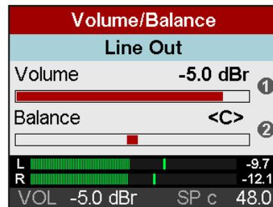
A push on encoder 2 (T) sets Balance to center (<C>)
