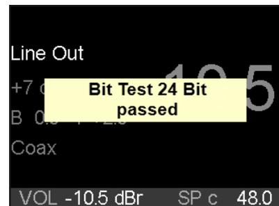
RME provides several audio files as free download: 44.1, 96 and 192 kHz in 16 bit, 24 bit and 32 bit. These files in WAV format can be played easily on Windows, Mac OS X and Linux. For ease of use (looping, players with fade in/out), the files contain the bit pattern several times. Runtime is about 4 seconds.
