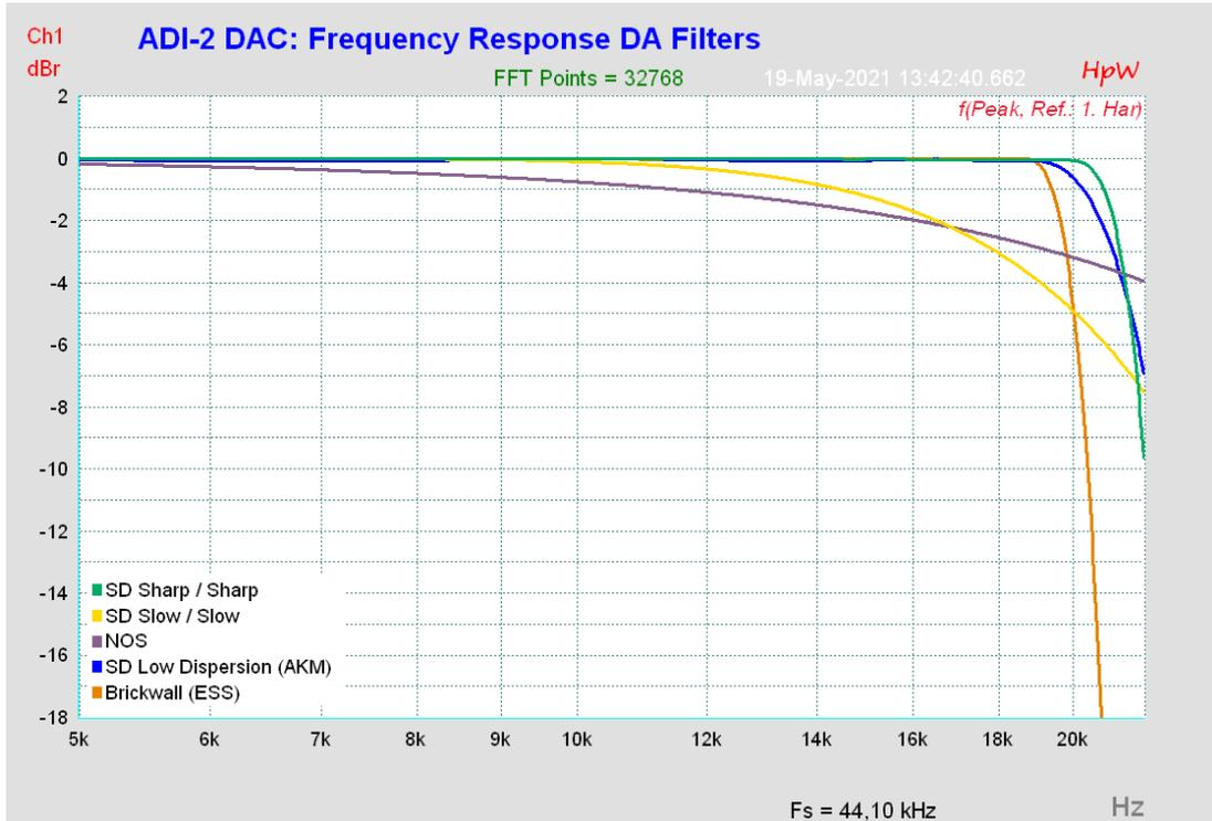
Notes: Sharp/SD Sharp and Slow/SD Slow are congruent. NOS shows a very early drop. SD Low Dispersion only in AKM chip units. Brickwall only in ESS chip units.
