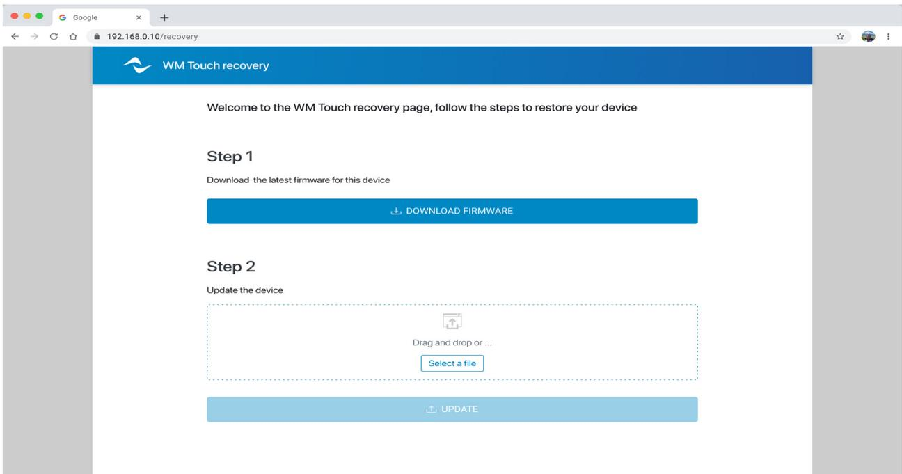
2. If the computer is connected to the internet, it will be possible to download the latest firmware version (Step 1). Alternatively, you can manually upload a file containing the firmware update (Step 2).
