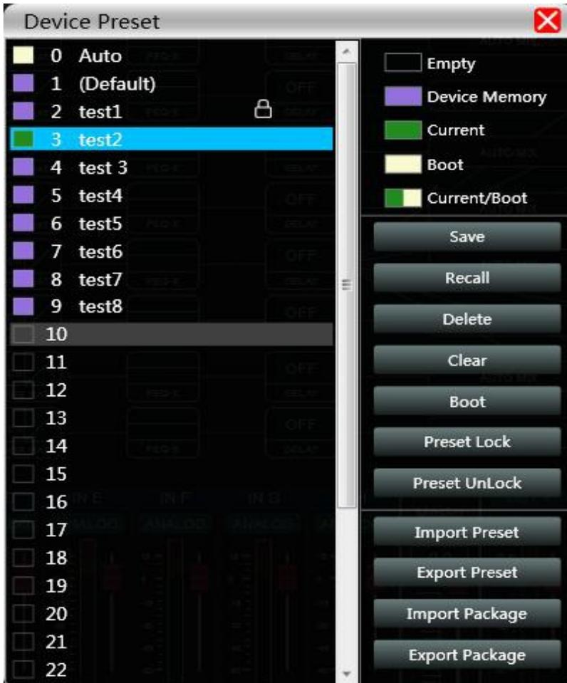
As shown in the figure above, the left side of the archive interface shows gears, where "0 Auto" is the system gear and cannot be used directly; "1 (Default)" is the default gear of the device, which can only be recalled, but cannot be deleted or overwritten. After recalling, all the device parameters will be restored to the factory default parameters; other gears can be freely saved, recalled, deleted, etc.
