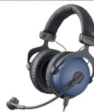
Headset with condenser microphone for use in loud environments.
