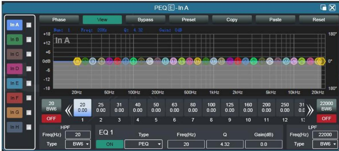
Phase: display the phase curve of the current channel.
