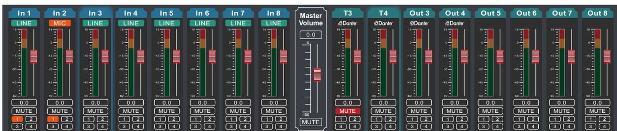
It can display the level, gain, input mode, channel name and other information of each channel, control the main switch of corresponding channel gain and mute, and turn on the group link function of input and output channels, so as to realize more powerful and convenient operation.
