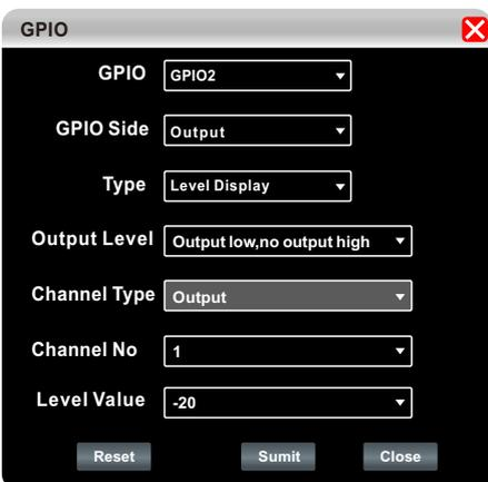
2. For example: when set GPIO side to output, as shown in the left figure, click "Submit" below to make it effective. When the electrical level of "output channel 1" reaches -20 dB, the same effect can be obtained by changing the output electrical level type, channel number and electrical level threshold.
