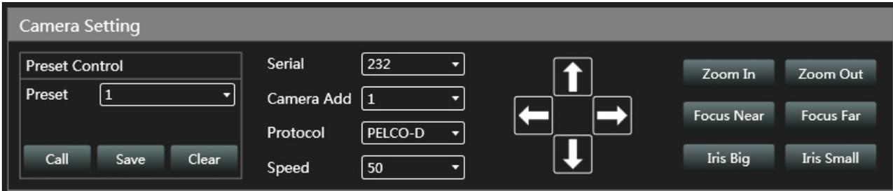
The camera setting is a camera debugging interface. Generally, the camera position is adjusted before the tracking starts, and finally the parameters of this part will remain on the camera.
