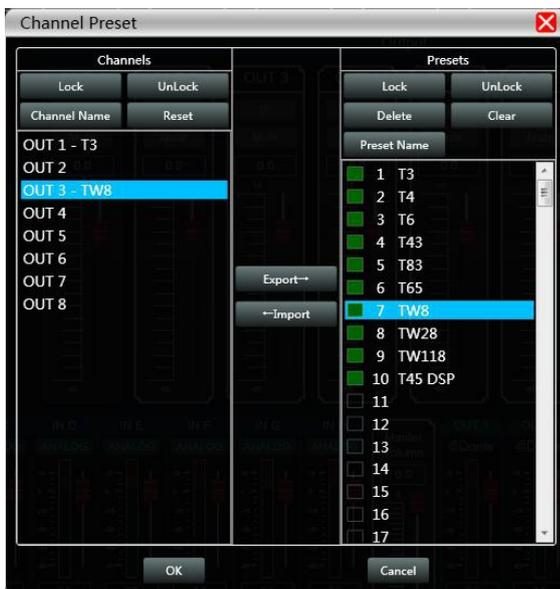
As shown in the picture, there are 8 output channels on the left, you can choose to save the preset for each channel through the "Export" key. You can also load the preset from the right output channel to any other output channel with the "Import" key. Encryption management is available for the presets (only for output EPQ and LIMIT encryption).
