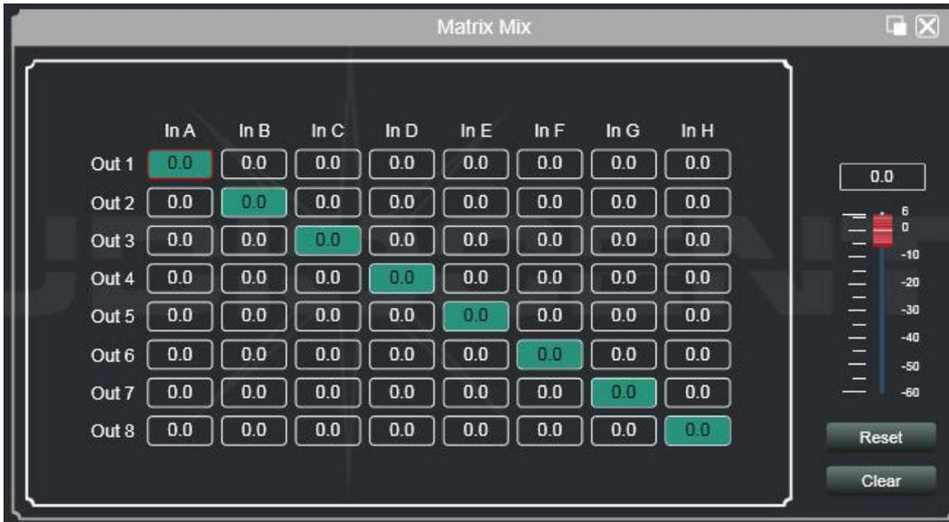
In the figure above, the left is output channel, and the upper is input channel. The value box with the value is the input / output channel mixing key. When the mixing key is green (double-click the value box to switch the state), signals of input and output channel realize the mixing function.
