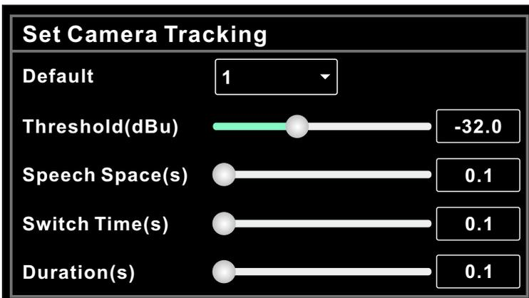
Default: when all mics have no input, turn the camera to the position set by default mic or send the association command defined by default mic.
