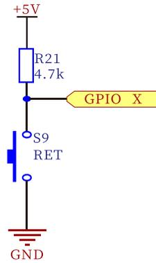
For the method of generating rising edge, the circuit schematic diagram is shown in the figure on the right. +5V can use output 5V from GPIO V port. GPIO X represents the GPIO port that you want to operate. A touch switch is connected in the middle. When you press the switch, a rising edge is generated.
