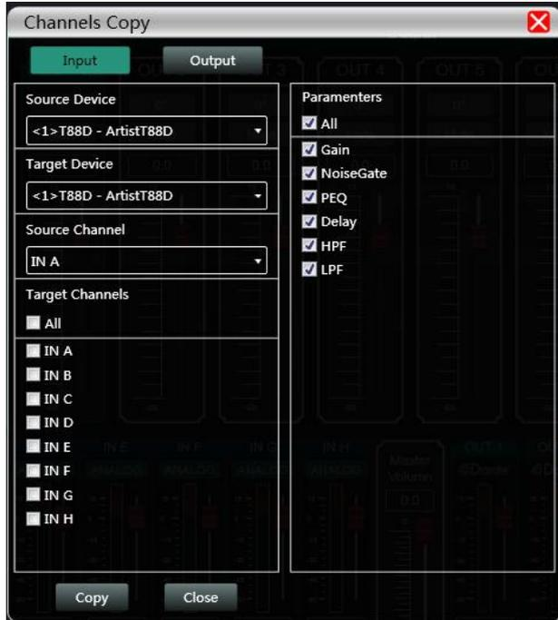
As shown in the figure above, channel copy is to select the channel parameters of one source device and copy them to the target channel of other target devices. Input channels and output channels cannot be copied with each other. The left side is the corresponding channel, and the right side is the copied parameters. The "Input" and "Output" buttons at the top of the interface can switch the channel type of the copy.
