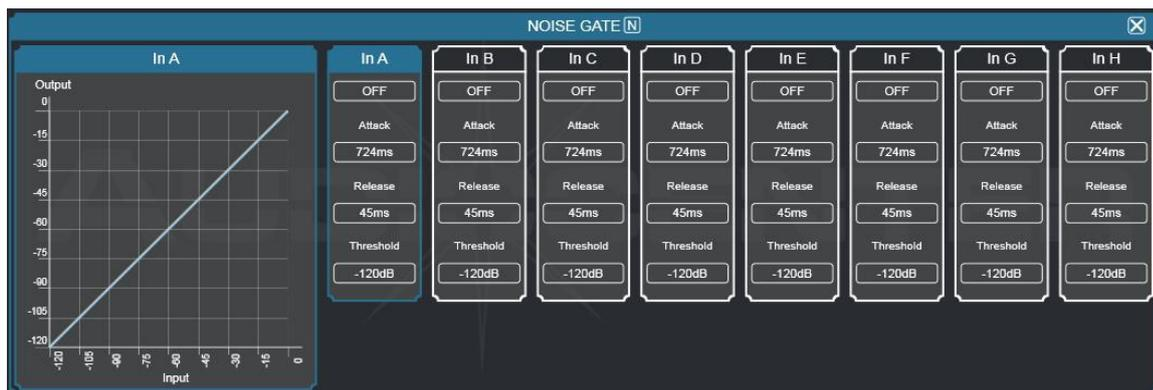
As shown in the figure above, click the noise gate switch **ON** to turn on or off the function of the noise gate of the channel. Green means turn on and red means turn off.
