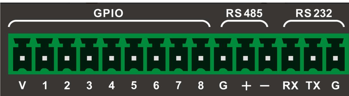
V: means 5V, the internal stabilized voltage output of the device, DC 5V 600mA
