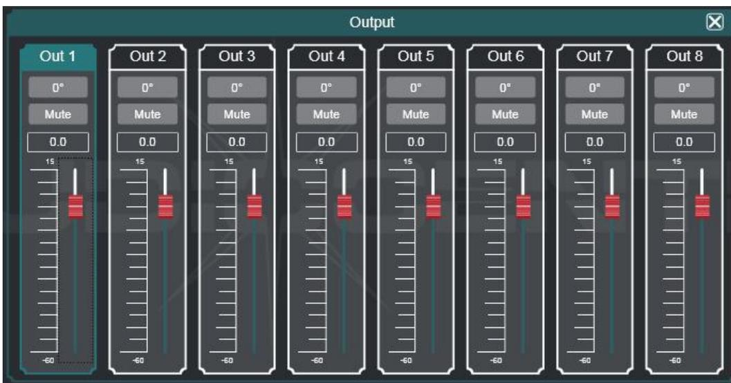
As shown in the figure above, the polarity and mute setting of the corresponding output channel can be controlled.
