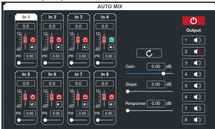
**0.0** is the input mixing gain of the corresponding channel. Drag the slider or input the corresponding value in the value box at the top; channel input mixing switch **⏻** and mute switch **🔇** control whether it is effective (red means off, green means effective); You can adjust the priority of the channel 0-10 to control PR value. The highest priority is level 10.
