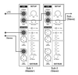
The BM9S II can be used stand-alone or together with multiple subwoofer units. Using multiple units may be helpful if the listening room is quite large or has difficult acoustic conditions. When using two or more subwoofers, the first one (designated "Master") controls the following subs (designated "Slave") via a subwoofer cable.
