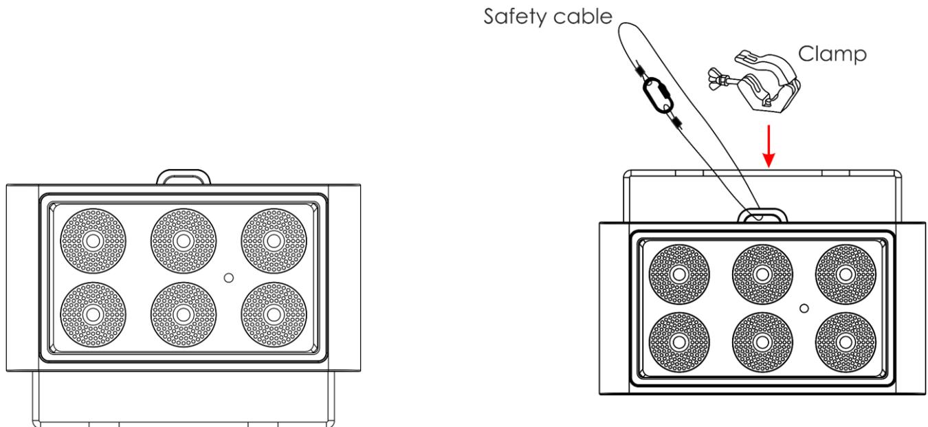
The Cameleon Flood 6WW can be placed on a flat stage floor or mounted to any kind of truss with a clamp.
