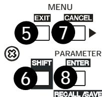
The left and right MENU keys (5, 7) allow to scroll through the different pages of the unit's setup menus.
