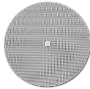
The versatile CMX20DT 8" two-way built-in loudspeaker produces a deep and warm sound ideal for speech and music. When using the loudspeaker at 16 ohms, you can connect up to 4 loudspeakers in parallel on each channel of a standard 4 ohms amplifier.
