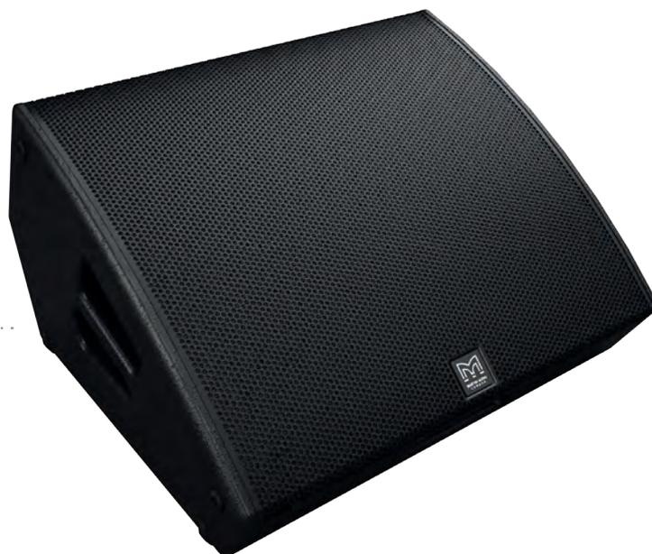
Combining very high output capability with Martin Audio's signature sonic performance and consistent coverage, the LE200 is the ultimate, everyday professional monitor. Its Coaxial Differential Dispersion drive unit comprises a powerful 15" (380mm)/3" (75mm) voice coil LF driver and a 1.4" (35mm) exit HF compression driver with a 3" (75mm) pure titanium diaphragm.
