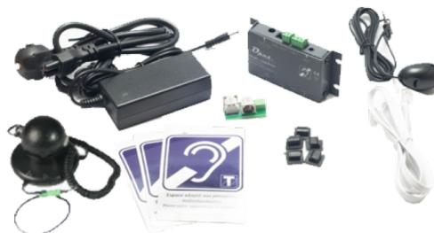
The DCL20-E is an induction loop kit that can be used to equip counters or reception desks. The set is designed to offer accessibility to hearing impaired people equipped with a hearing aid with the T position but also for non-hearing instrument hearing aids though the OP-E headphones.
