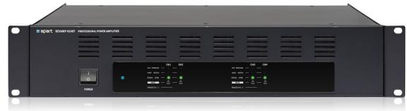
REVAMP4240T is a professional 4-channel digital power amplifier with 4 x 240 watt output power @ 100 volt, but the unit is also bridgeable to 2 x 480 watts @ 100 volt. The unit incorporates a high efficient SMPS power supply and outputs with efficient Class D output topology.
