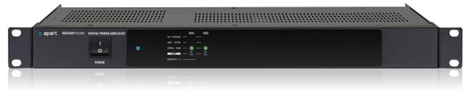
Immaculate sound performance, extremely reliable, maintenance-free this is how we would describe our latest REVAMP2120T. This 2-channel digital power amplifier provides 2 x 120 watts output power @ 100 volts or @ 4 ohms, that can easily be bridged into a powerful 240 watts @ 100 volts or 8 ohm single amplifier. The REVAMP2120T is a convection cooled class-D amplifier without built-in fans which implies that the amplifier is completely noiseless and dust-free at all times.
