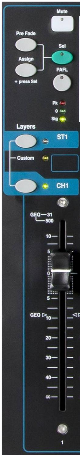
**Mute key** – Press to turn off the channel audio signal. This affects the send to all mixes including LR, effects and stage monitors. The Mute key lights red when the channel is muted. It flashes when it is muted by a Mute Group master.
