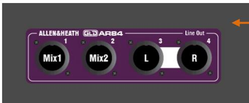
The screen presents a picture of the AR84 rack output sockets to show which Qu signals are mapped.
