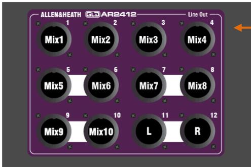
The screen presents a picture of the AR2412 rack output sockets to show which Qu signals are mapped.
