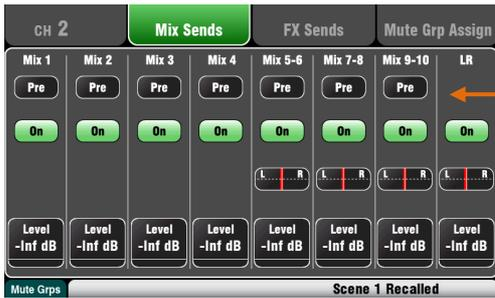
Each send can be set **Pre** or **Post** fader. It is typical to set monitor sends pre-fade so that the channel fader does not affect the monitor mixes, and to set effects and fill speaker sends post-fade so that their levels do follow the faders.
