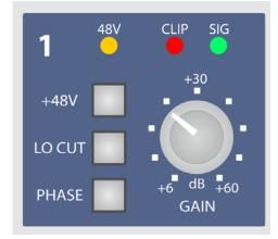
+48V (switch) activates phantom power. Phantom power should only be activated when using condensor microphones which require such a power supply, and only on the specific channel. Another important rule: plug-in the microphone first, then switch on the phantom power. The QuadMic will apply the voltage smoothly (soft start). In case the microphone is plugged in while phantom power is already switched on, a current peak (spike) is generated that can destroy the sensitive microphone input stages.
