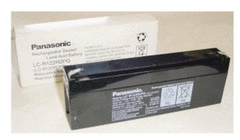
We tested a Panasonic LC-R122R2PG battery, 12 V 2.2 Ah, which can operate the QuadMic for 4 hours. Measuring the voltage while discharging shows that the QuadMic remains completely in working order even shortly before the battery voltage collapses (7 Volts.)
